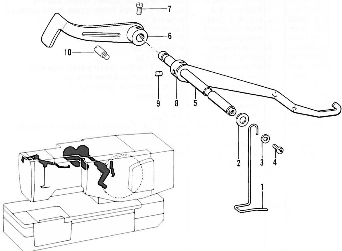
Q. 下軸関係 / Lower shaft mechanism / Untere Welle /
