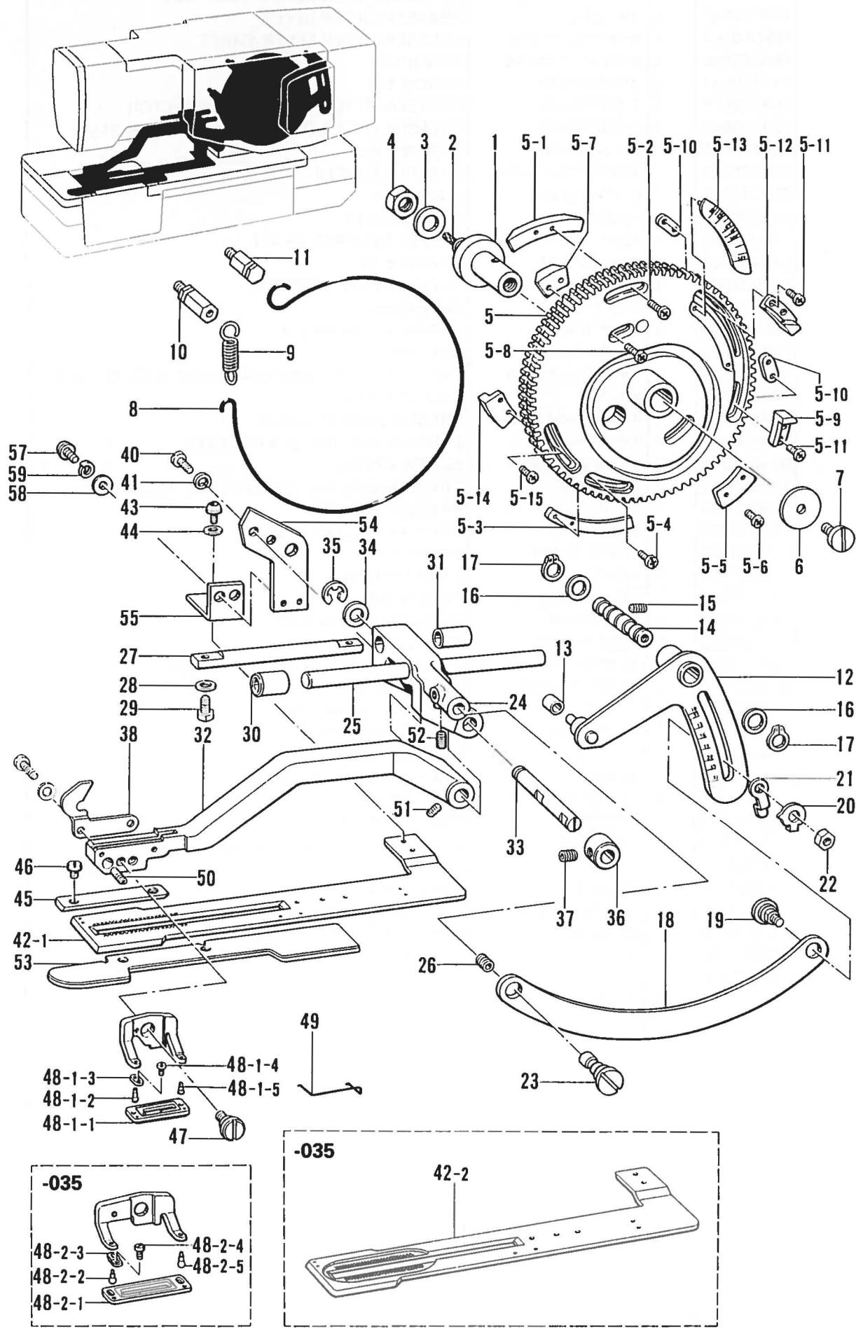
M. 送り関係 / Feed mechanism / Transportvorrichtung /
