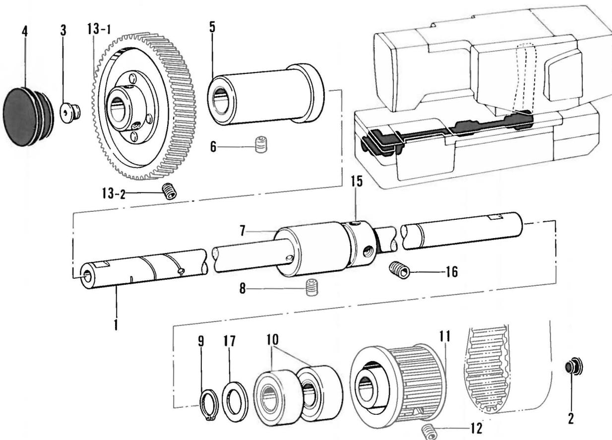
P. 糸切れ感知関係 / Thread breakage detector mechanism / Fadenbruchfühler /
